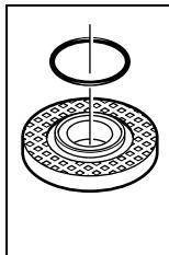
**Mounting flange for grinding spindle M 14:** A plastic part (O-ring) is fitted around the centring collar of mounting flange 10. If the O-ring is missing or damaged, the mounting flange 10 must be replaced before resuming operation.
