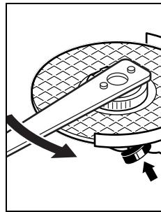
A properly fastened, undamaged quick-clamping nut can be manually loosened by turning the knurled ring in an anticlockwise direction.
