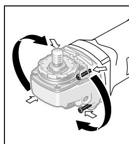
The machine head can be rotated with respect to the machine housing in 90° steps. In this manner, the On/Off switch can be brought into a more convenient position for special working situations, e.g. for left-handed persons.
