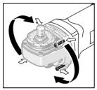
The machine head can be rotated with respect to the machine housing in 90° steps. In this manner, the On/Off switch can be brought into a more convenient position for special working situations, e.g., for cutting operations using the cutting guide with dust
