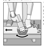
The machine must always work in an upgrinding motion. Otherwise, the danger exists of it being pushed **un-controlled** out of the cut.
