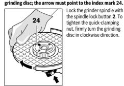
Lock the grinder spindle with the spindle lock button 2. To tighten the quick-clamping nut, firmly turn the grinding disc in clockwise direction.
