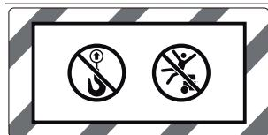
**Do not hang the vacuum cleaner on a crane hook, e.g. in order to transport it.** The vacuum cleaner is not suitable for moving with a crane. There is a risk of injury and damage if you do this.
